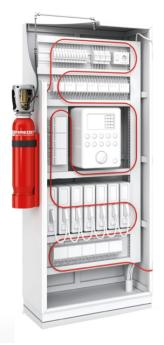
We have designed a Tube Based Fire Suppression System to fight with fire that occur in the "micro-environment" of electric panels. This system is a self-activating suppression system that reliably suppresses fires in seconds. This system uses polymer heat sensing tube that will rupture when exposed to a flame. This specialized detection tubing combines leak resistance, flexibility, durability and precise temperature sensitivity, allowing it to react quickly when the heat from a fire is present.
